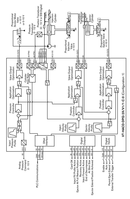
Typical injection circuit using one proportional control valve, one proportional ejector valve and the PLC to control output AO2 (Out2) directly to a proportional screw motor valve.
