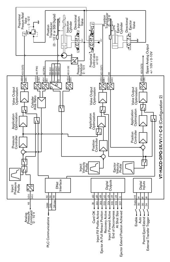
Injection circuit using one proportional flow control valve for injection velocity, ejector velocity and screw motor speed in combination with a separate proportional pressure control valve. Output AO3 (Out3) can be configured so the PLC directly controls the analog output for other functions that can be unrelated to the injection control.
