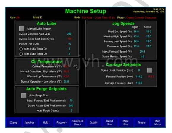
The machine setup screen can only be accessed from the Process Overview/Main Menu screen. This screen has a variety of information on it pertaining to lubrication, oil temperature, jogs, carriage and purging. To make Machine setup even easier, all setpoints are saved to the current recipe.
