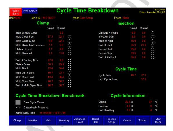
The cycle time breakdown screen is accessed from the Process Overview/ Main Menu screen. This screen provides the time in seconds at which each machine phase completes.
