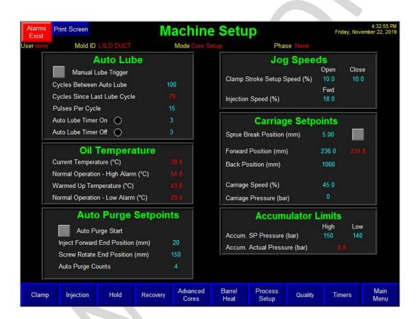
The machine setup screen can only be accessed from the Process Overview/Main Menu screen. This screen has a variety of information on it pertaining to lubrication, oil temperature, jogs, carriage, purging and accumulators.
