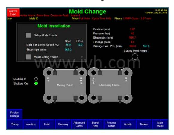
The Mold Change screen can be accessed from the production setup screen. This screen provides a visual display of the status of the mold clamps and cylinders. The cylinders are indicated unlocked or locked by the green indicator.
