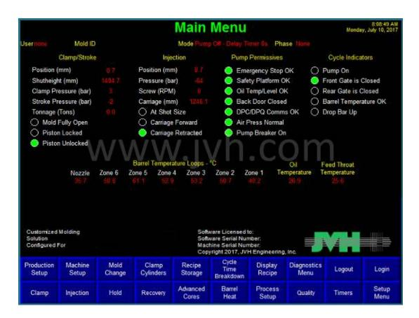
The Process Overview screen is designed to give the user a simple overview of the machine status. This screen includes all relevant temperatures, positions, pressures and indicators for basic press operation. It is also the main hub from which many other screens are accessed. The buttons in the bottom row appear on all other profile screens allowing one-touch access to all profile parameters. The buttons on the top row exist on this screen only.
