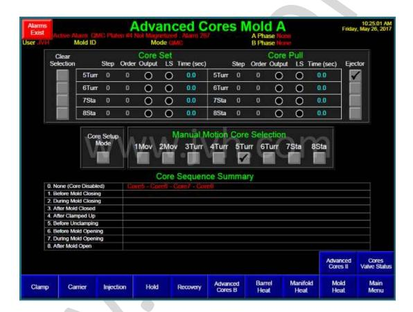
The Advanced Cores screen is the first of two core screens and is found by touching the Advanced Cores button from any of the profile screens. The advanced core screen can be utilized to configure nearly any sequence of core operation.
