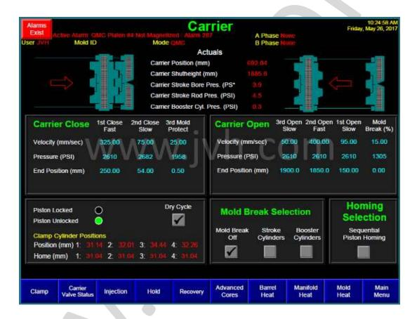
The Carrier screen provides all information required to configure the camp open and close profiles
