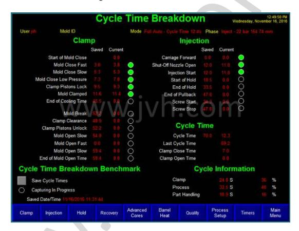
The cycle time breakdown screen is accessed from the Process Overview/ Main Menu screen. This screen provides detailed information about when each process of the cycle has begun during the cycle.
